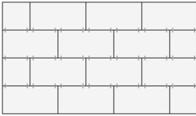
/Correct installation of tiles with plastic pins/
