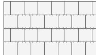
/Correct installation of tiles with plastic pins/
